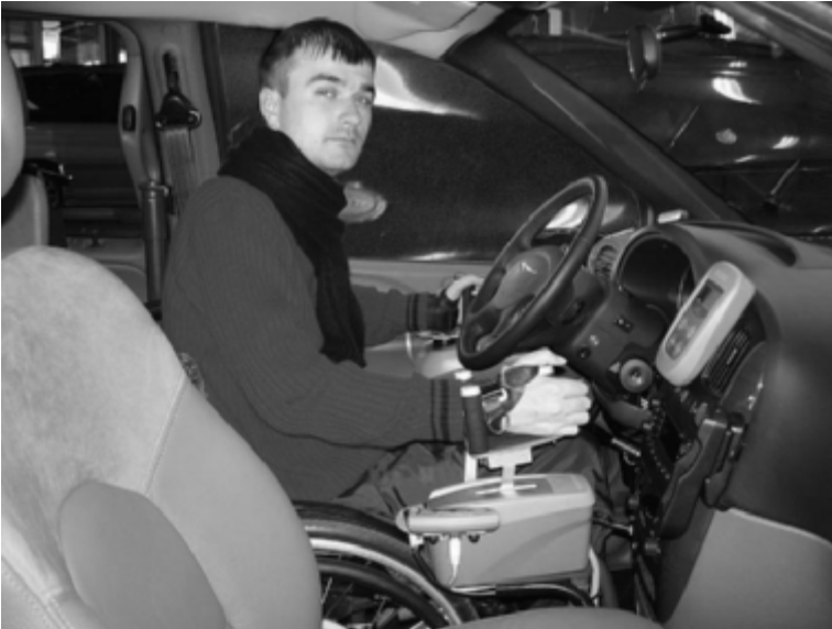
Illustration 15: Systems which are purely steer-by-wire or drive-by-wire are already in use in the construction of specialist vehicles for drivers with limited mobility. They are configured as redundant systems and have TÜV approval. The left hand steers a mini steering wheel and the right hand operates the throttle (Source: Paravan Ltd.)
