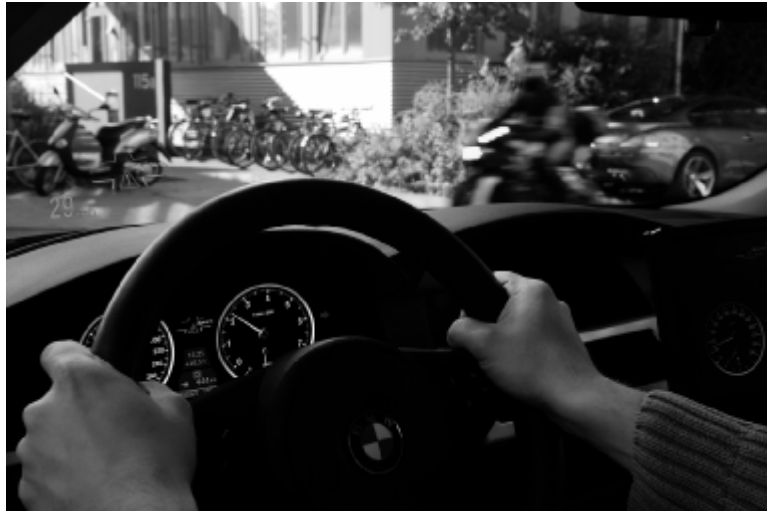
Illustration 20: The assistant for traffic from side roads uses a head-up display on the windscreen to warn of moving objects outside the driver's direct field of vision (Source: BMW Group)
