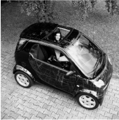
Illustration 4: The homogeneous, high-quality appearance of the roof module on the Smart is made possible by using multilayered plastic films (Source: BASF)
