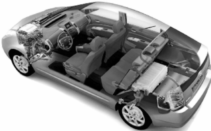
Illustration 9: View inside a Toyota Prius: the electric motor is next to the combustion engine, the battery behind the back seat (Source: Toyota)
