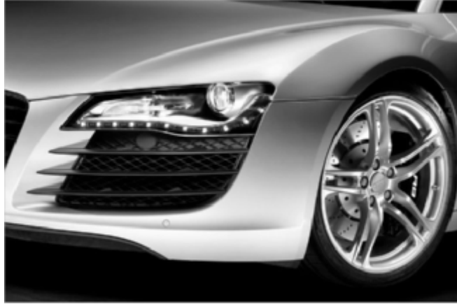
Illustration 22: The first LED-only headlamp with 54 LEDs in the Audi R8 (Source: Audi)
